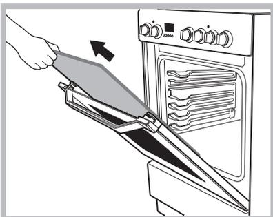
5. Remove the glass sheet and do the cleaning as indicated in chapter: „Care and maintenance”.
