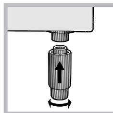
If it is necessary to level the appliance, screw the adjustable feet into the positions provided on each corner of the base of the cooker (see figure).
